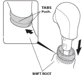
Pry out on the bottom of the shift knob cover and 3. remove the cover.
