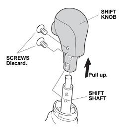
Install the new select knob using the two new screws. Using a torque screwdriver, torque the screws to 1.57 N⋅m (14 lb-in). Do not overtighten the screws.
